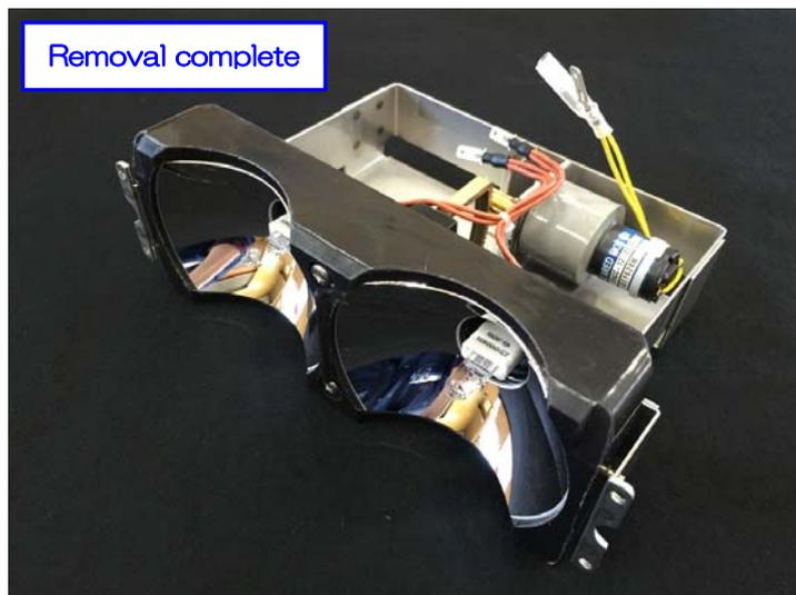
**B. [Replace with LED module to power head.]**
